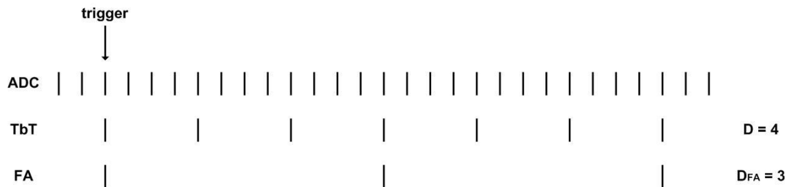
Figure 59: Phase of ADC, turn-by-turn and FA transmissions relative to the trigger.
